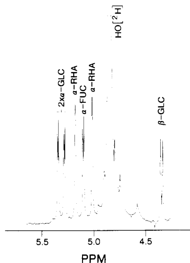
FIGURE 3: The 360-MHz ^1\text{H} NMR of Ose-1. The oligosaccharide, derived from LOS-1 by deacylation with NaOH, was dissolved in ^2\text{H}_2\text{O} . \text{HO}^2\text{H} was set at 4.74 ppm.
